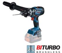
Part no. 0 601 9J5 1L0 Battery voltage 18 V Torque (soft/hard/max.) 84/100/150 Nm No-load speed (1st / 2nd gear) 0 - 550 / 0 - 2,200 rpm Max. impact rate 30,000 bpm 1.5 / 13 mm Chuck capacity, min./max. Weight excl. battery 2.2 kg
