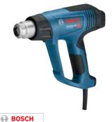
**Technical Specifications** HSN code 84672900 0 601 2A6 2F0 Part no. Power input 2,000 W Temperature range 50-630°C Adjustable temperature Yes steps 150 - 500 litre/min Air flow rate Durability 600 h Weight 0.65 kg
