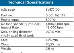
Scope of supply: MRP: ₹ 16,100 Auxiliary handle; Chuck key;
